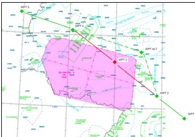
Fig. 6. Re-routing due to a TRA [DFS]
