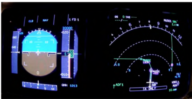
Figure 4: Primary Flight Display and Navigation Display [source: Technical University Berlin].
