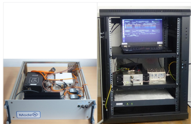
Figure 13: Mode N aircraft system (l) and ground station (r).
