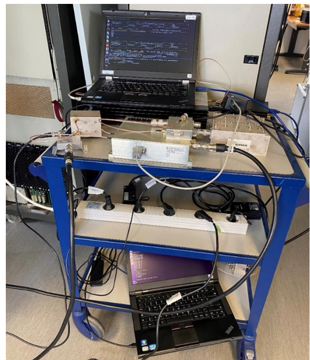
Figure 2: Structure of the Mode N TX/RX (on top) and Mode N RX (below) ground stations with notebooks as processing units.
